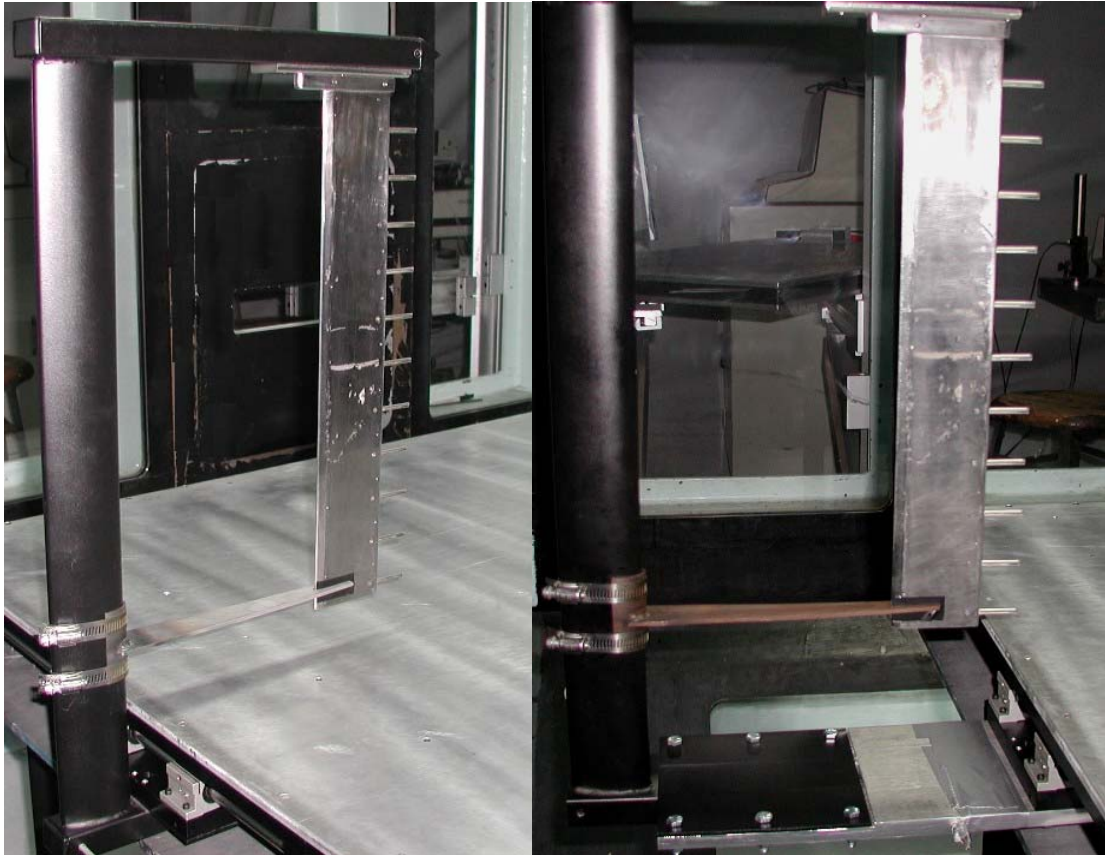
Figure 7. Comparison of Pressure Rake at Nominal & Extended Positions
