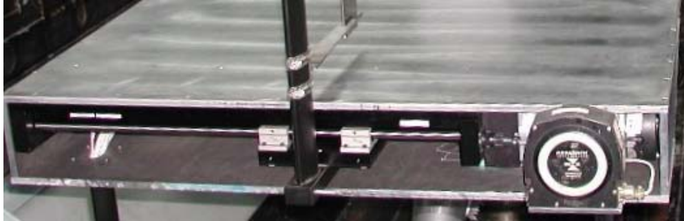
Figure 5. Aft View of Transverse Used for Pressure Rake
